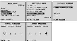
After entering your passcode, you will be prompted to enter the items you want to limit. When the thermostat has been locked out, the passcode must be entered to change any of the items that have been locked or to enter the MAIN MENU of the thermostat. The thermostat relocks when it returns to the main operating display. "LOCKED" appears in the display Message Center when a thermostat has been locked out.
