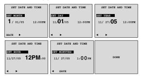
**NOTE:** When installed with an Aprilaire® Model 6504, the time setting will be set on all the thermostats on the system.
