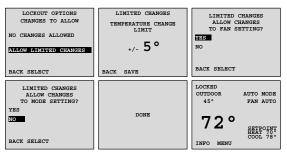
To permanently unlock the thermostat, enter the passcode to get into the SETTINGS MENU, then select UNLOCK from the LOCKOUT OPTIONS menu.
