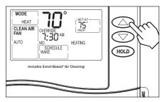
**Press** or to immediately adjust the temperature. This will temporarily override the temperature setting for the current programmed time period. The new temperature setting will be maintained until the next time period of the programmed schedule.
