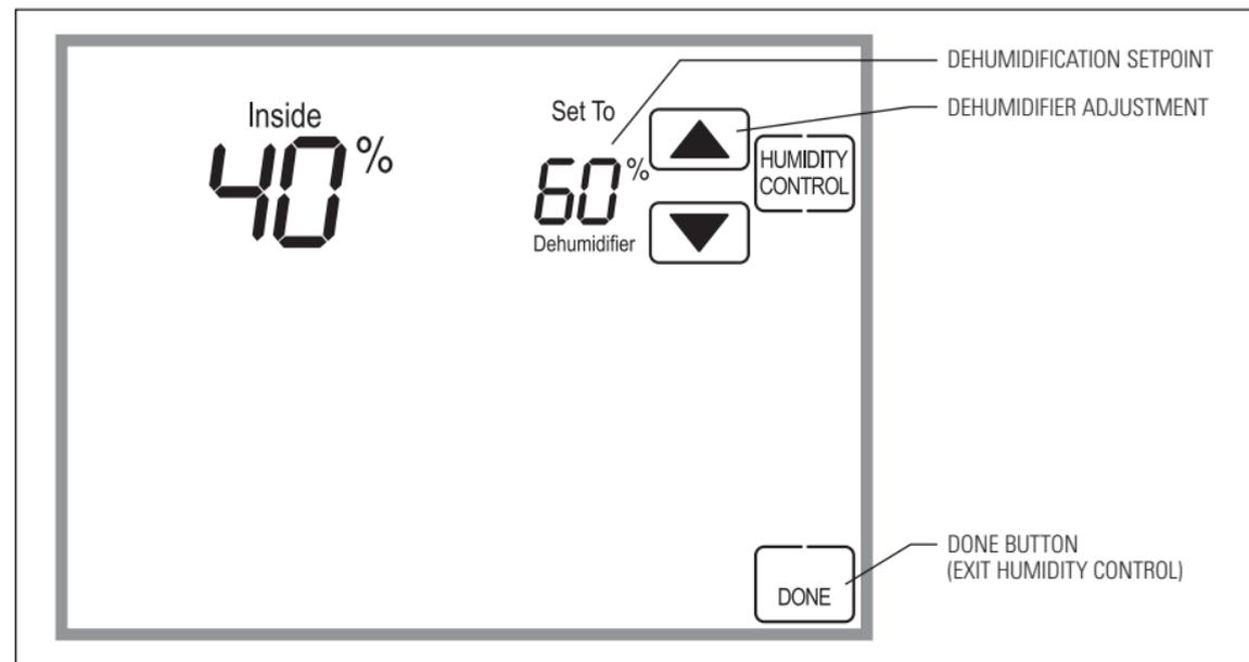
**If dehumidification is done with the air conditioner**, the thermostat will cool up to 3°F beyond the cooling setpoint for dehumidification. Note overcooling may not be sufficient to meet the dehumidification setpoint.
