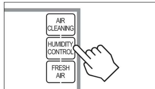
The Humidity Control screen is used to access control for both humidification and dehumidification.
