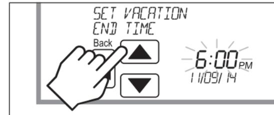
**Press [DONE]** to save and exit, Or **[CANCEL]** to exit without saving. The thermostat will save and exit if nothing is pressed within 20 seconds.
