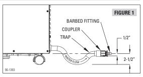
Screw the supplied hose barb fitting into the coupler and attach the supplied 1/2 inch I.D. drain hose.
